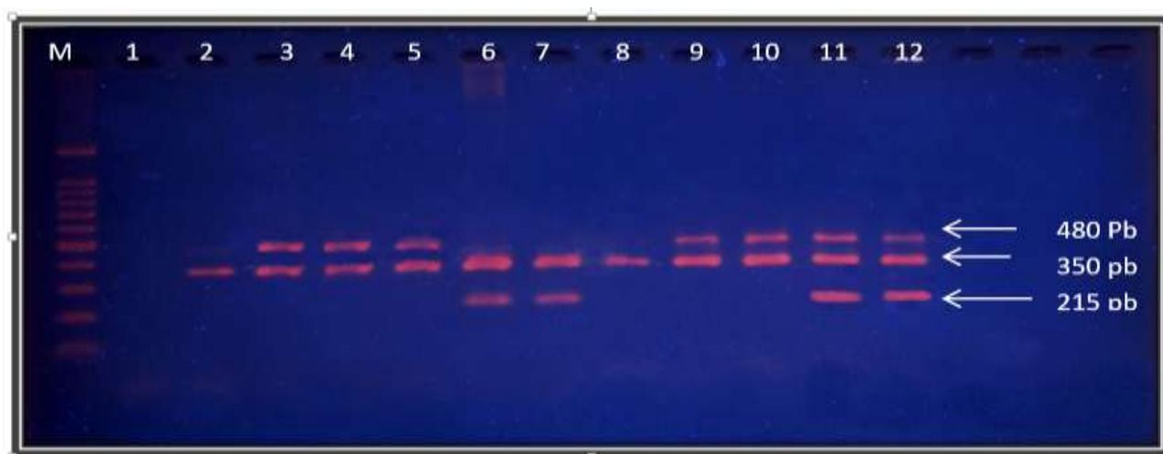
Fig. 1. Multiplex PCR products analyzed on 2% agarose gel. The presence or absence of GSTM1 and GSTT1 genes was detected by the presence of a band at 215 bp (corresponding to GSTM1) and a band at 480 bp (corresponding to GSTT1). A band at 350 bp (Corresponding to albumine gene) was always present and was used as an internal control to document successful PCR amplification. Lanes 1, a negative control. Lane 2,8 individuals with null alleles for both GSTM1 and GSTT1 genes showing only one band at 350 bp corresponding to the internal control (albumine gene fragment). Lanes 3,4,5,9,10 individuals with GSTT1 present (480 bp) and GSTM1 null alleles. Lanes 6 and 7: individuals harboring GSTT1 null and GSTM1 present (215 bp) alleles. Lanes 11, 12 individuals with both GSTT1 and GSTM1 alleles present. M is a DNA molecular marker (100bp).
